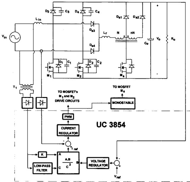
Fig. 7. Simplified circuit of the implemented prototype.
