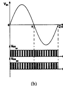
Fig. 4 (a) Topological stages for the second operation mode. (b) Gate signals of the MOSFET's for the second operation mode.
