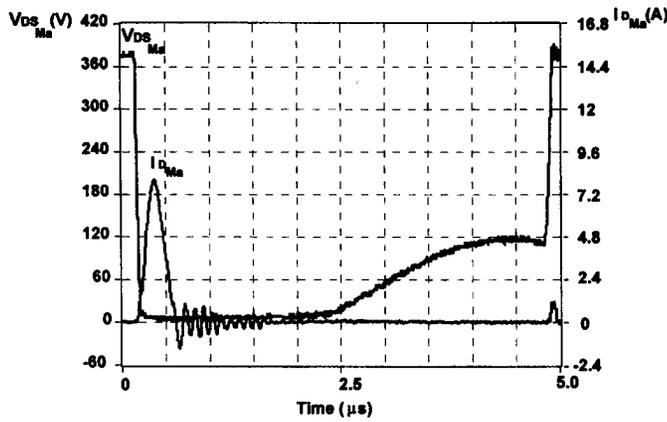
Fig. 10. Commutation detail in the auxiliary MOSFET  $M_a$ .
