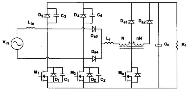
Fig. 2. Power stage diagram of the proposed converter.
