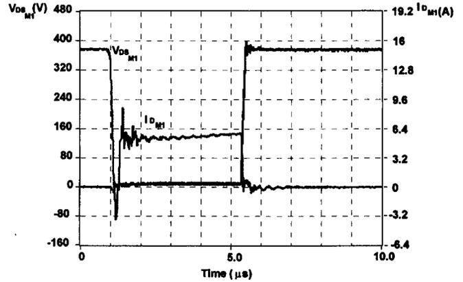
Fig. 9. Commutation detail in the main MOSFET  $M_1$ .
