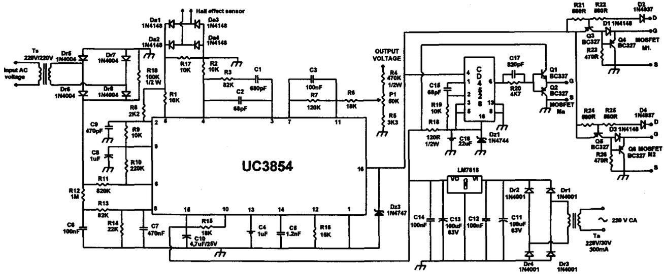
Fig. 14. Complete control circuit of the proposed converter.
