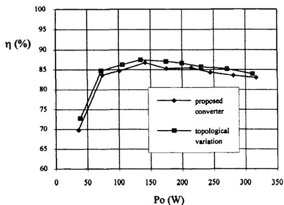
Fig. 17. Efficiency curves.
