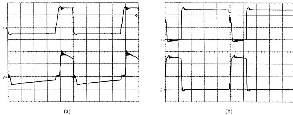
Fig. 11. Experimental waveforms. (a) Voltage [50 V/div.] across the secondary side of the transformer and current [10 A/div.] through capacitor  $C_b$ . (b) Voltage [20 V/div.] across the rectifier diodes; upper trace odd diodes and lower trace even diodes. Time scale [5  $\mu$ s/div.].
