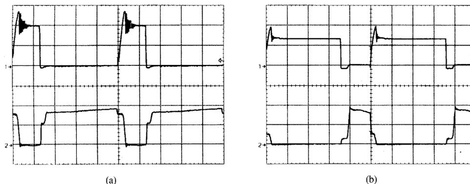
Fig. 14. Experimental results of the topological variation. (a) Voltage [100 V/div.] and current (5 A/div.) through switch  $S_1$ . (b) Voltage [50 V/div.] and current (5 A/div.) through switch  $S_2$ . Time scale [5  $\mu$ s/div.].
