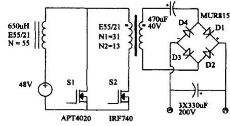
Fig. 9. Power stage diagram of the implemented converter.
