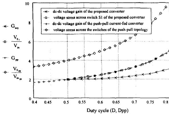
Fig. 6. Graphical comparison between asymmetrical PWM dc-dc converter and push-pull, current-fed topology.
