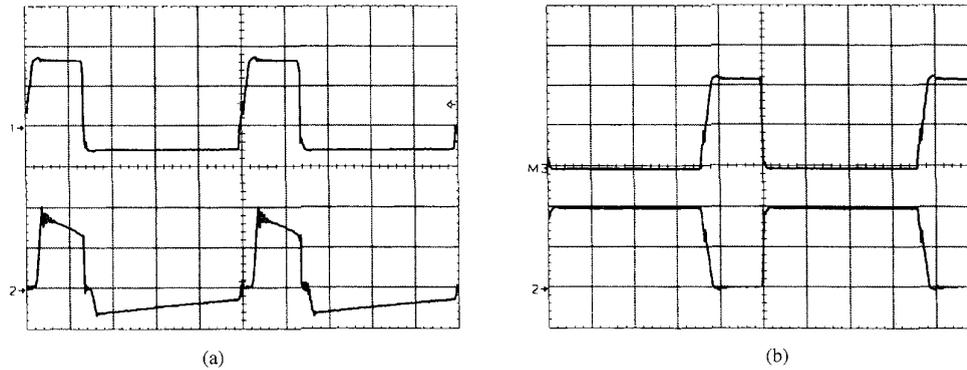
Fig. 15. Experimental waveforms. (a) Voltage [50 V/div.] across the secondary side of the transformer and current [10 A/div.] through capacitor  $C_b$ . (b) Voltage [50 V/div.] across the rectifier diodes, upper trace  $D_r$  and lower trace  $D_b$ . Time scale [5  $\mu\text{s}/\text{div.}$ ].
