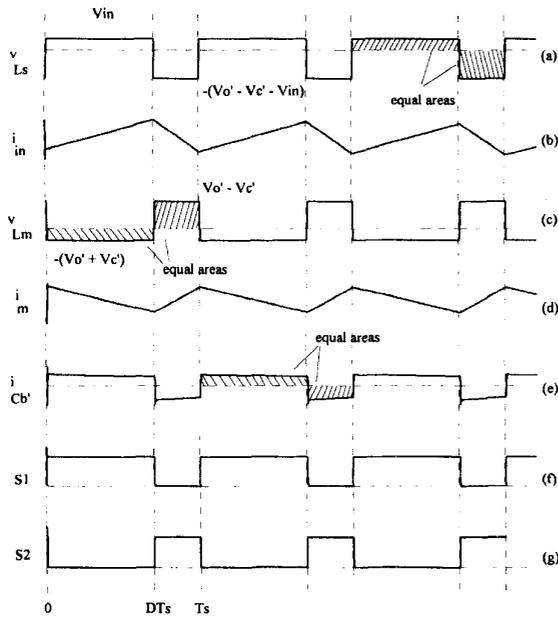
Fig. 5. Typical theoretical waveforms presented by the asymmetrical PWM dc-dc converter operating in mode I (continuous conduction).
