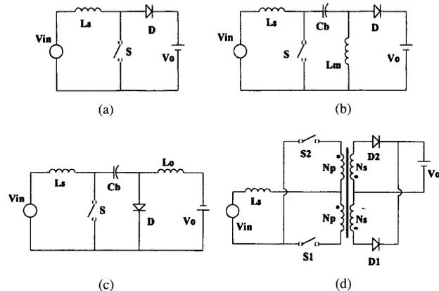
Fig. 1. Four basic current-fed converters: (a) boost, (b) sepic, (c) cuk, and (d) push-pull.
