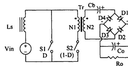
Fig. 2. The proposed current-fed, isolated PWM dc-dc converter.
