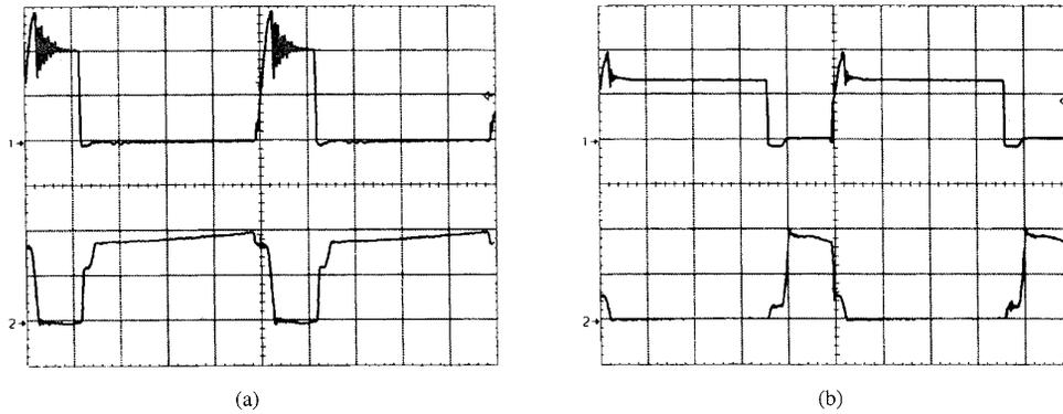
Fig. 10. Experimental waveforms. (a) Voltage [100 V/div.] and current [5 A/div.] through switch  $S_1$ . (b) Voltage [50 V/div.] and current [5 A/div.] through switch  $S_2$ . Time scale [5 s/div.].
