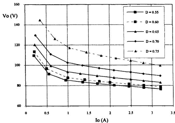
Fig. 16. Experimental characteristics of the topological variation.
