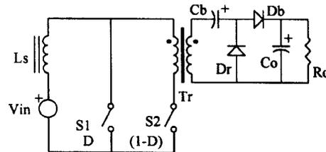
Fig. 13. Topological variation of the proposed PWM dc-dc converter.
