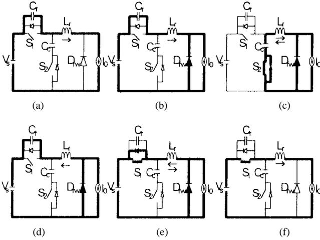
Fig. 13. Topological stages assumed by Buck-buck-boost converter.
