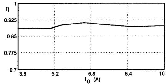
Fig. 21. Experimental curve of efficiency with different load conditions and nominal duty cycle.
