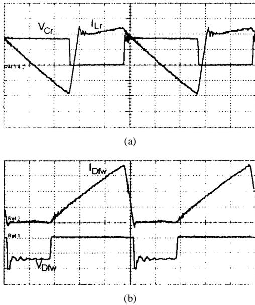
Fig. 19. (a) Voltage across  $C_r$  and current through  $L_r$ . (b) Voltage across  $D_{fw}$  and current through  $D_{fw}$ ; (voltage: 100 V/div; current: 5 A/div; time scale: 2  $\mu$ s/div).
