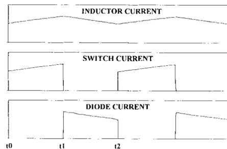
Fig. 14. Main-current waveforms in a switching period.
