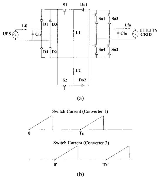
Fig. 18. Two converters operating in DCM  $180^\circ$  shifted.
