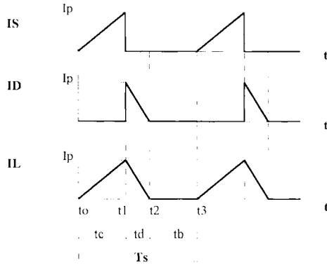
Fig. 8. Main waveforms in a switching period.
