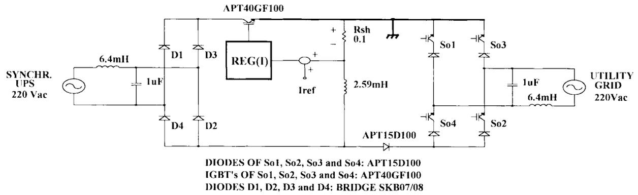
Fig. 15. Implemented circuit for CCM.
