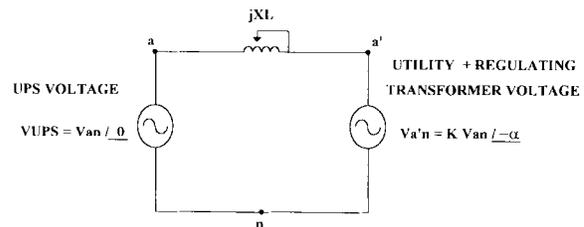
Fig. 3. Equivalent circuit diagram of proposal in [4].
