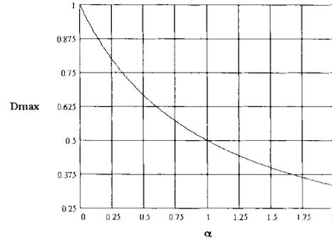
Fig. 9. Maximum duty cycle for DCM operation.
