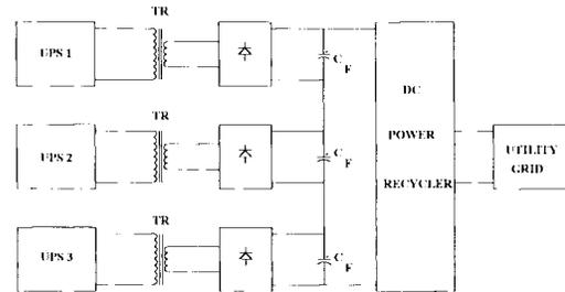
Fig. 1. Block diagram of proposal in [1] and [2].
