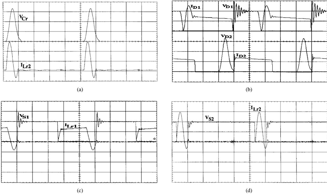
Fig. 8. (a) Voltage across  $C_r$  and current through  $L_{r2}$ . (b) Voltages and currents through  $D1$  and  $D2$ . (c) Voltage across  $S1$  and current through  $L_{r1}$ . (d) Voltage across  $S2$  and current through  $L_{r2}$  at full load. Time scale:  $10 \mu\text{s}/\text{div}$ ; voltage:  $200 \text{ V}/\text{div}$ ; current:  $5 \text{ A}/\text{div}$ .
