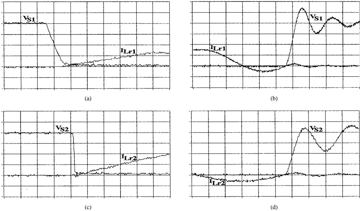
Fig. 9. Details of experimental waveforms for the new ZCS-PWM boost converter at full load. Voltage:  $100 \text{ V}/\text{div}$ ; current:  $5 \text{ A}/\text{div}$ . (a) Time scale:  $200 \text{ ns}/\text{div}$ . (b) Time scale:  $1 \mu\text{s}/\text{div}$ . (c) Time scale:  $200 \text{ ns}/\text{div}$ . (d) Time scale:  $400 \text{ ns}/\text{div}$ .
