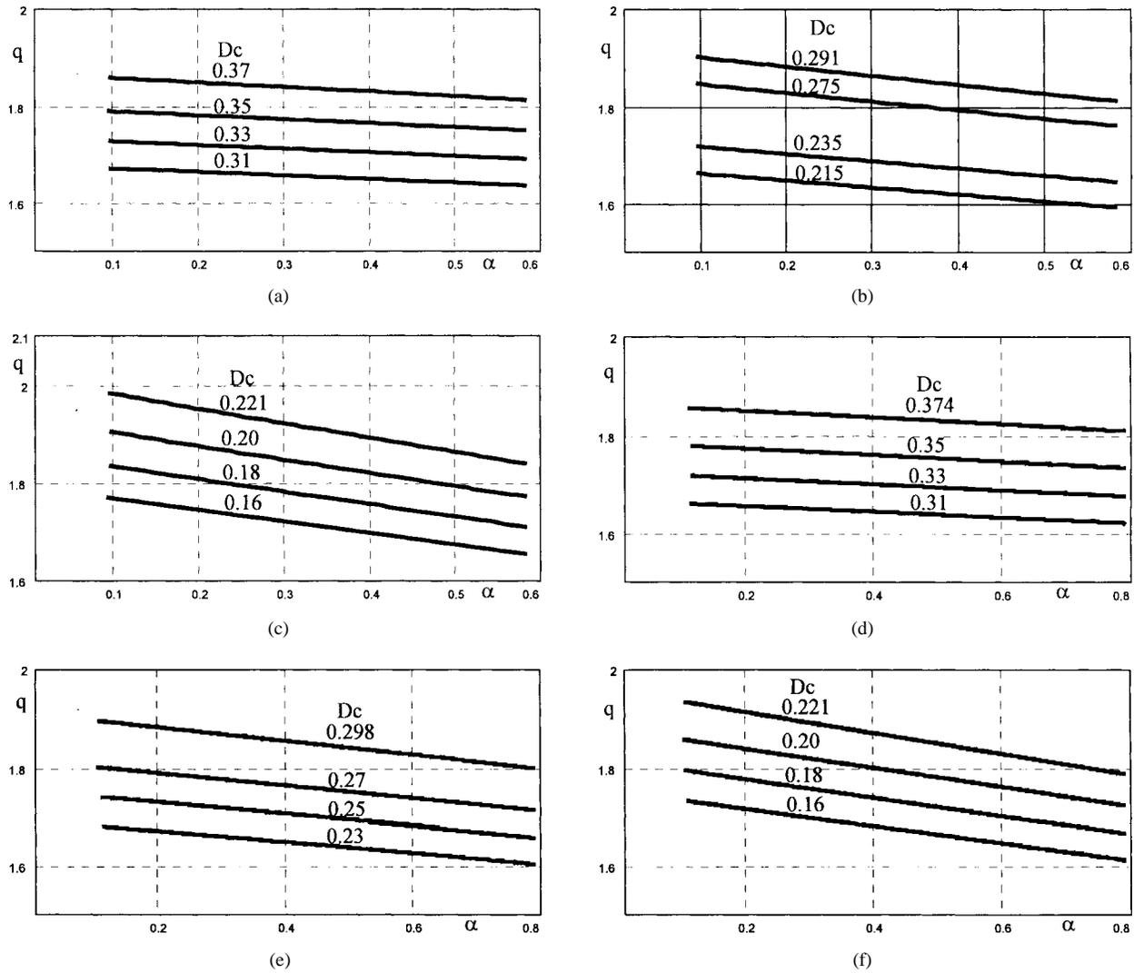
Fig. 6. Theoretical output characteristics for the new ZCS-PWM boost converter. (a)  $\beta = 0.6$  and  $f = 0.1$ . (b)  $\beta = 0.6$  and  $f = 0.2$ . (c)  $\beta = 0.6$  and  $f = 0.3$ . (d)  $\beta = 0.8$  and  $f = 0.1$ . (e)  $\beta = 0.8$  and  $f = 0.2$ . (f)  $\beta = 0.8$  and  $f = 0.3$ .
