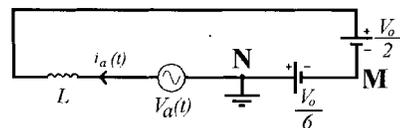
Fig. 5. Equivalent circuit for  $i_a$  (phase "A" input current) during the  $30^\circ$ - $60^\circ$  stage.
