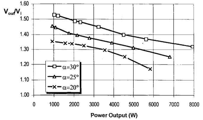
Fig. 11. Output characteristics of the 7.4-kW prototype.
