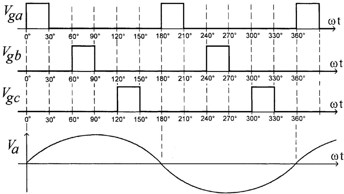
Fig. 2. The low-frequency switching pattern presented in [6].
