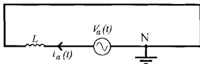
Fig. 4. Equivalent circuit for  $i_a$  (phase "A" input current) during the  $0^\circ$ - $30^\circ$  stage, when the switch  $S_a$  is gated on.
