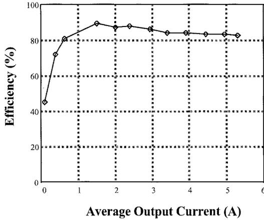
Fig. 12. Efficiency curve for the proposed converter.
