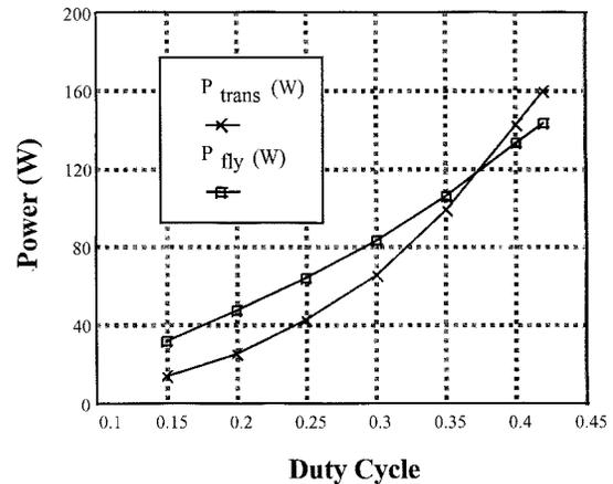
Fig. 15. Power sharing between transformer and flyback inductor.
