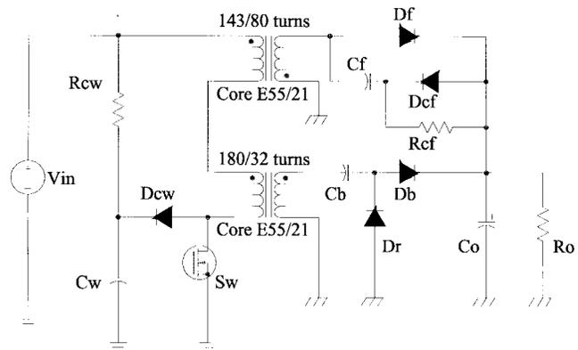
Fig. 10. Power stage diagram of the proposed converter.
