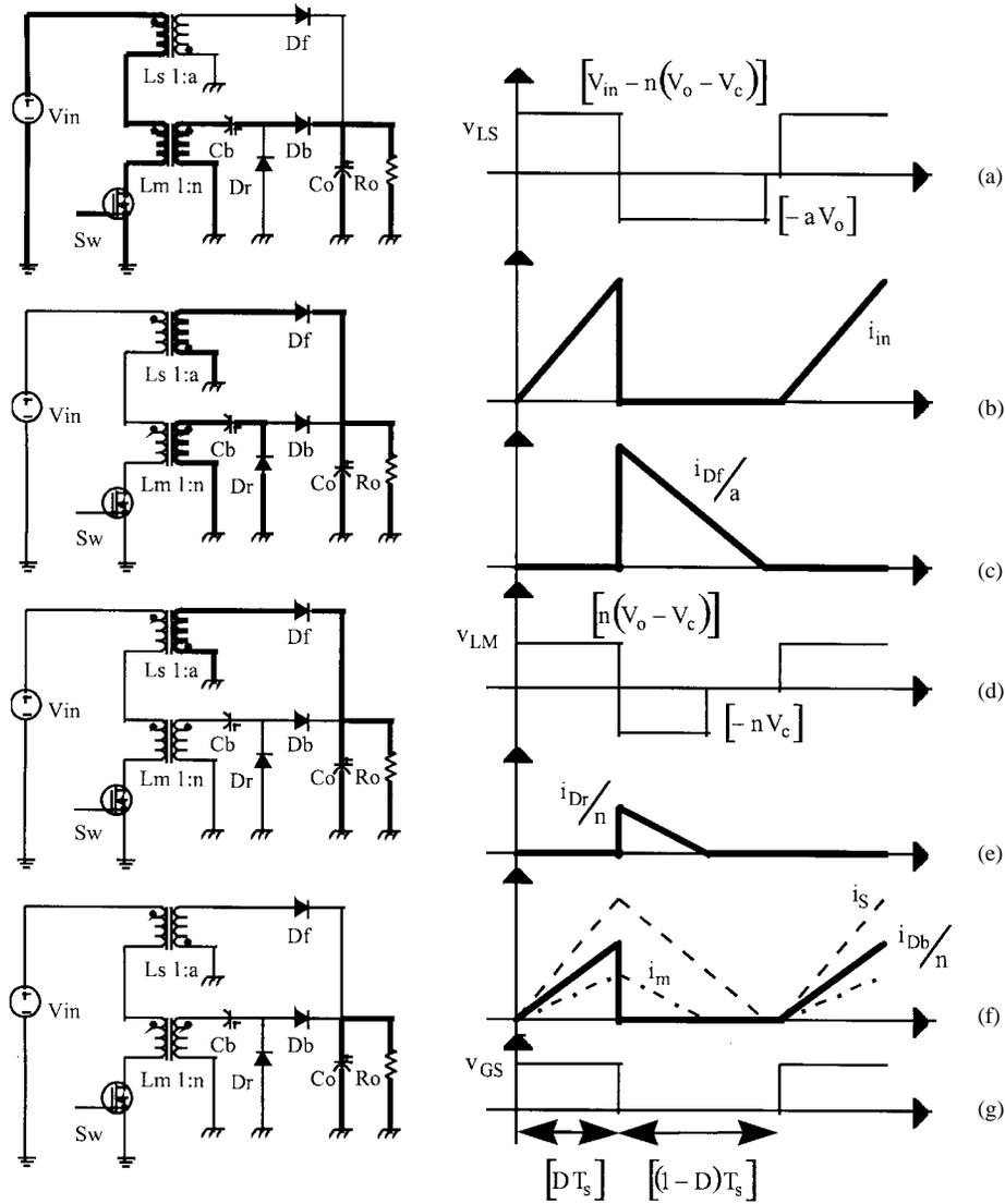
Fig. 8. Discontinuous conduction mode—case III.
