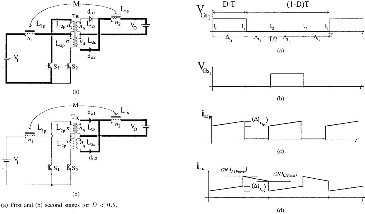
Fig. 2. (a) First and (b) second stages for  $D < 0.5$ .
