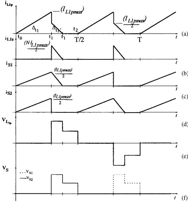
Fig. 9. Waveforms for the discontinuous conduction mode and  $D > 0.5$ : (a) current through the primary winding  $L_{1P}$ , (b) current through secondary winding  $L_{1S}$ , (c) current through switch  $S_1$ , (d) current through switch  $S_2$ , (e) voltage across the primary winding of the push-pull transformer  $L_{2p}$ , and (f) voltage across the switches.
