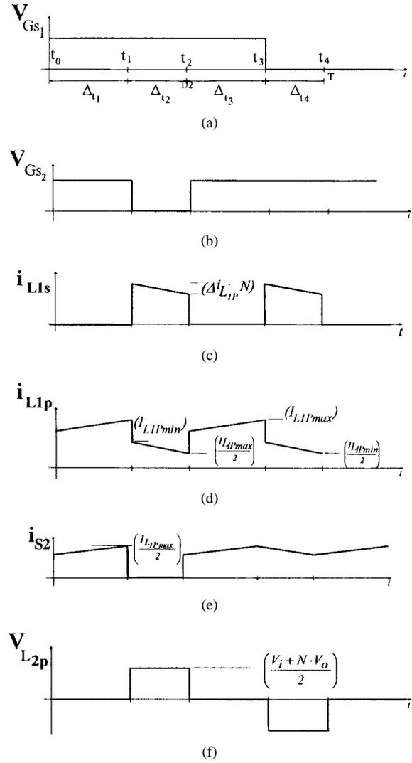
Fig. 8. Waveforms for the converter operating at  $D > 0.5$  in CCM: (a) and (b) driving signals of  $S_1$  and  $S_2$ , (c) current through the secondary winding  $L_{1S}$ , (d) current through the primary winding  $L_{1P}$ , (e) current through the switches, and (f) voltage across the primary winding of the push-pull transformer.
