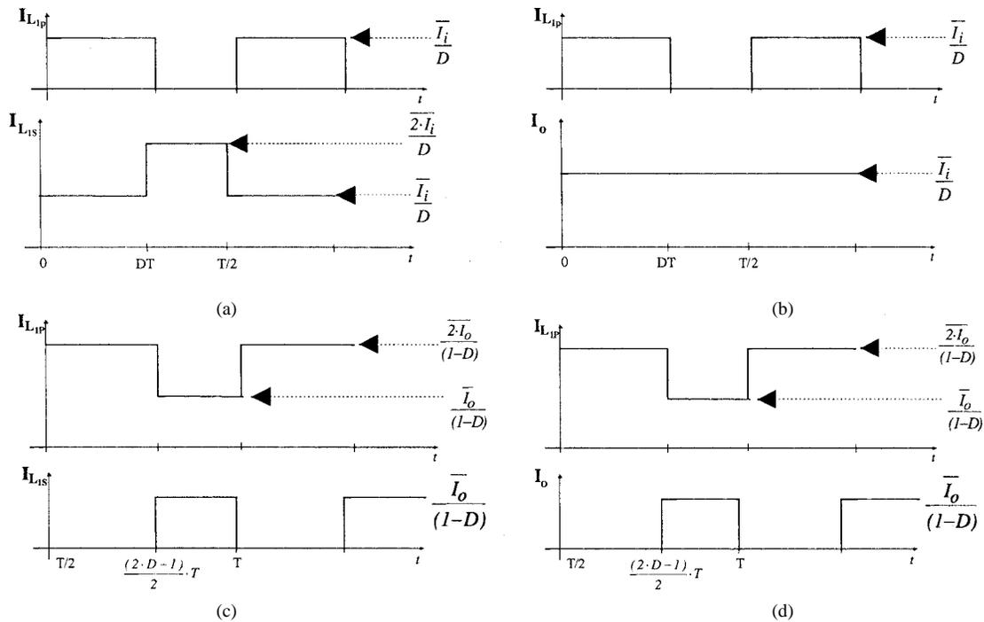
Fig. 15. Input and output currents with  $L_{1p} = L_{1s} = \infty$  and  $N_1 = N_2 = 1$ : (a) new converter with  $D < 0.5$ , (b)  $D > 0.5$ , (c) the conventional converter with  $D < 0.5$ , and (d)  $D > 0.5$ .
