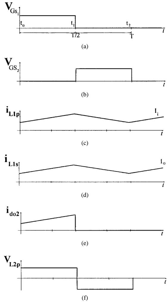
Fig. 6. Theoretical waveforms for the converter operating at  $D = 0.5$ : (a) and (b) driving signals of  $S_1$  and  $S_2$ , (c) current through the primary winding  $L_{1P}$ , (d) current through the secondary winding  $L_{1S}$ , (e) current through output diodes, and (f) voltage across the primary winding of the push-pull transformer.
