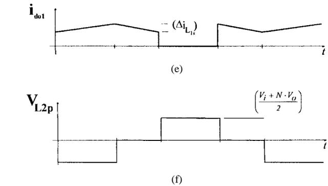
Fig. 3. Waveforms for the new converter working at  $D < 0.5$  in CCM: (a) and (b) driving signals, (c) input current, (d) current through the inductor  $L_{1s}$ , (e) current through the output diodes, and (f) voltage across the primary winding of the push-pull transformer.
