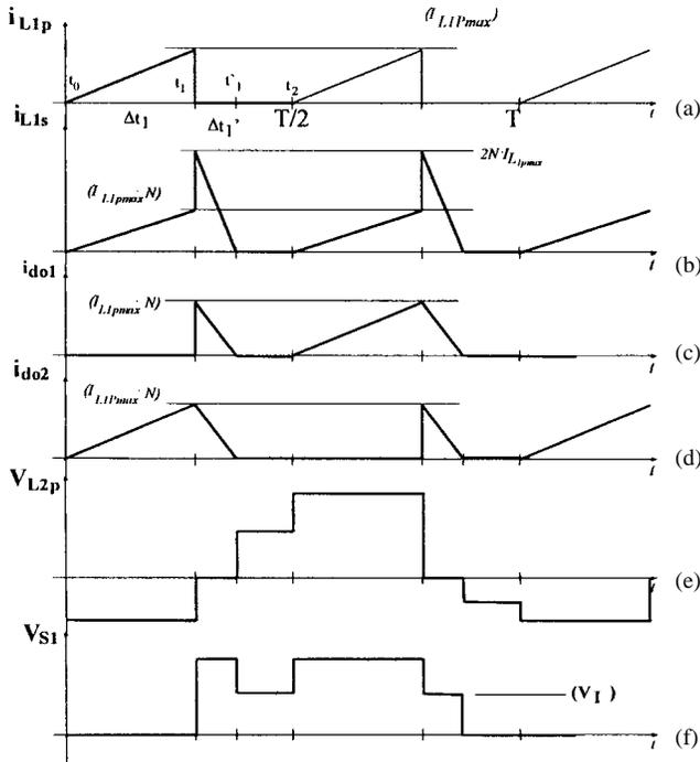
Fig. 4. Waveforms for discontinuous operation mode at  $D < 0.5$ : (a) current through the primary winding  $L_{1P}$ , (b) current through secondary winding  $L_{1S}$ , (c) and (d) current through output diodes, (e) voltage across the primary winding of the push-pull transformer, and (f) voltage across the switches.
