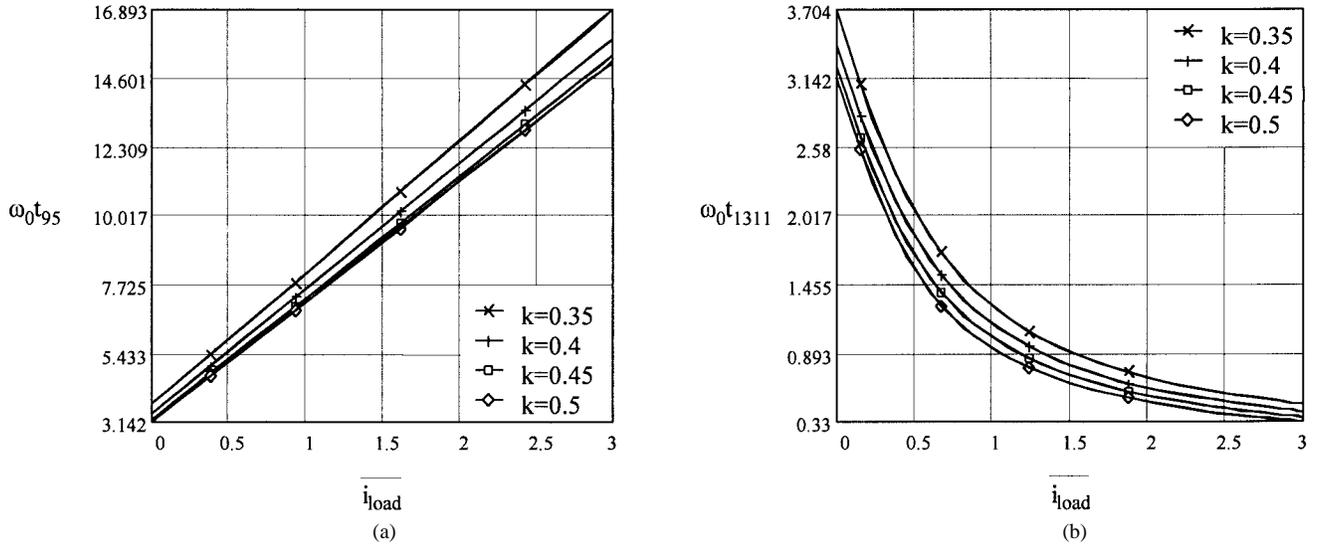
Fig. 8. Variations of commutation durations  $t_{95}$  and  $t_{1311}$  with load current and transformer ratio: (a) diode-to-switch commutation and (b) switch-to-diode commutation.
