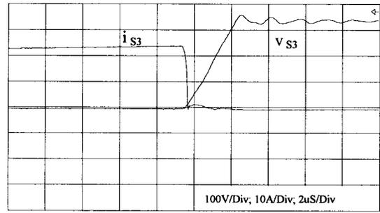
Fig. 16. Extended turn-off process of  $S_3$ .
