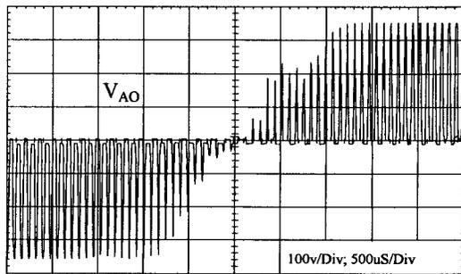
Fig. 13. Experimental inverter output voltage  $V_{AO}$ .
