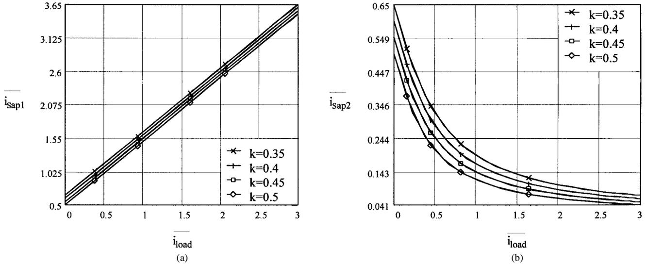
Fig. 9. Variations of the auxiliary switch peak currents with load current and transformer ratio: (a) diode-to-switch commutation and (b) switch-to-diode commutation.
