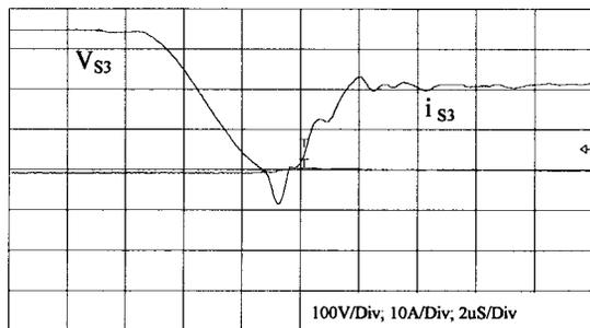
Fig. 15. Extended turn-on process of  $S_3$ .
