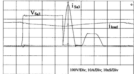
Fig. 17. ZCS commutation of the auxiliary switch ( $S_{a3}$ ).
