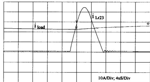
Fig. 19. Resonant inductor current waveform at  $i_{load} = 22$  A.
