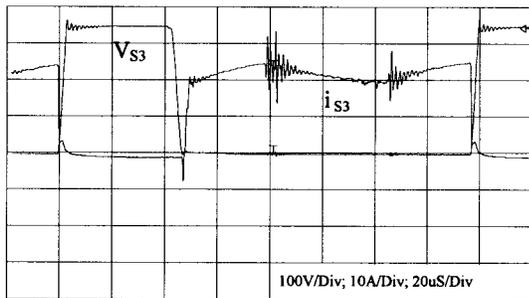
Fig. 14. ZVS commutation of the main switch ( $S_3$ ).
