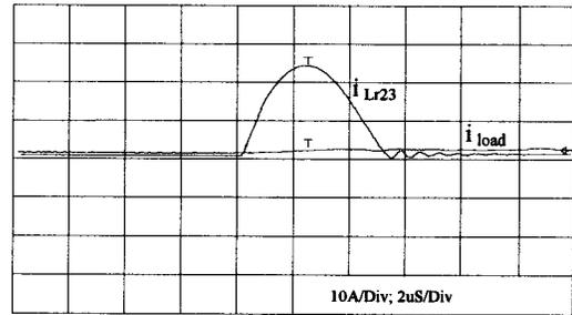
Fig. 18. Resonant inductor current waveform at  $i_{load} = 0$  A.
