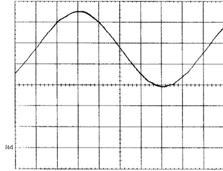
Fig. 17. Voltage across the capacitor  $C_1$  (50 V/div-2 ms/div).
