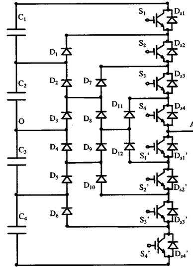
Fig. 3. Structure of the proposed new diode clamping inverter (five level).
