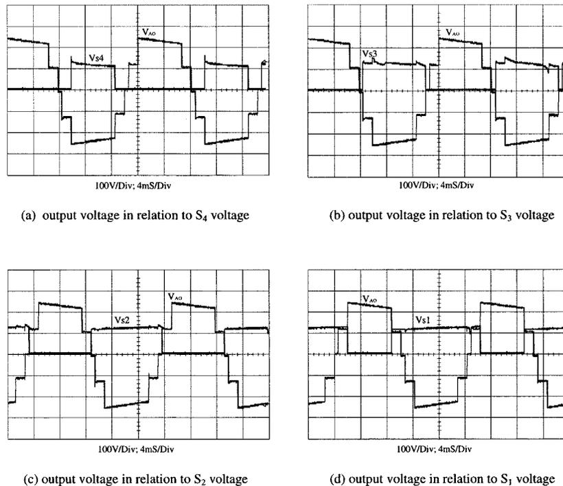
Fig. 12. Experimental output voltage of the new inverter in relation to the blocking voltages across  $S_4$ ,  $S_3$ ,  $S_2$ , and  $S_1$  respectively. Each main switch sees the nominal blocking voltage.
