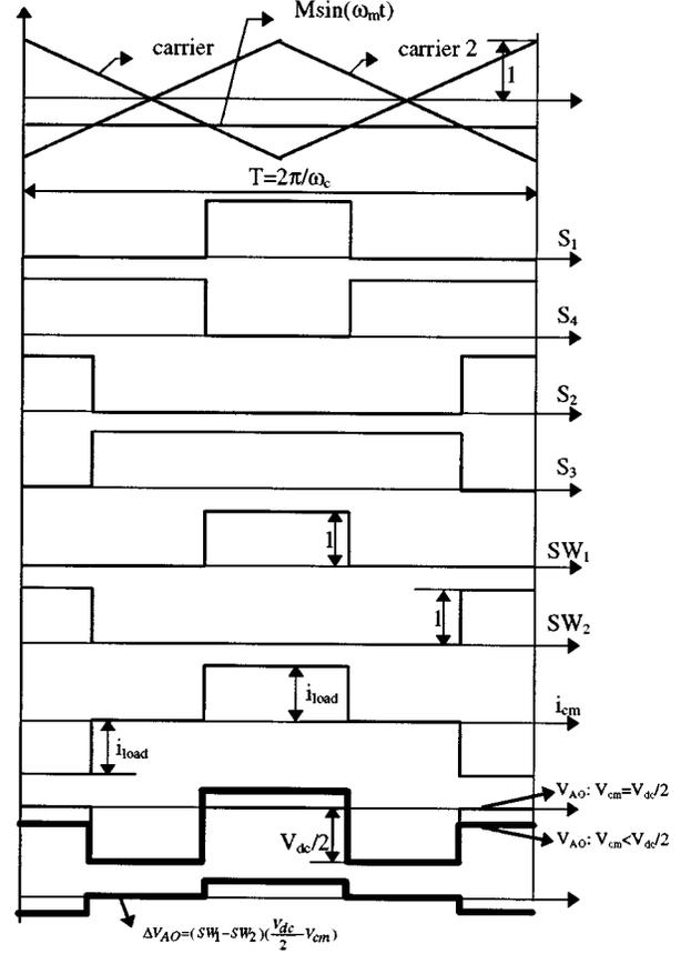
Fig. 2. Sub-harmonic PWM modulation for the half-bridge three-level capacitor-clamping-inverter, with load current in the positive direction.  $M$ : modulation index;  $\omega_m$ : modulating angular frequency;  $\omega_c$ : carrier angular frequency;  $T$ : switching period.
