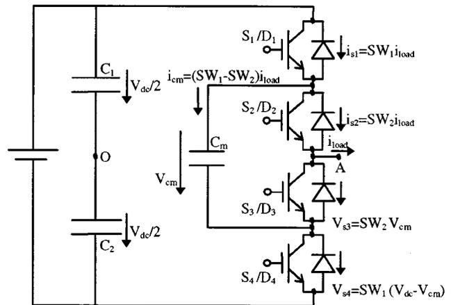
Fig. 1. Structure of a half-bridge three-level capacitor-clamping-inverter.
