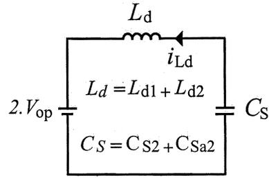
Fig. 20. Equivalent circuit of the auxiliary switch turn-off.
