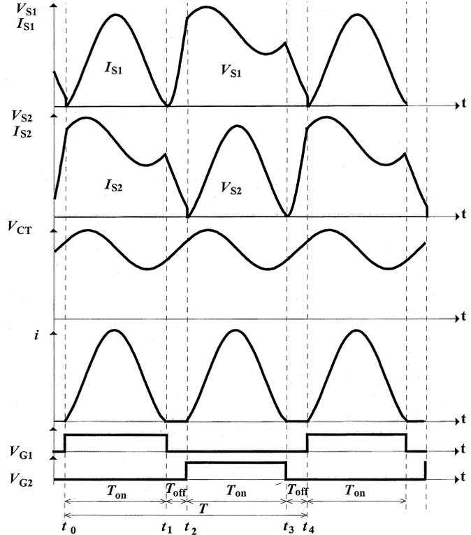
Fig. 5. Main theoretical waveforms.
