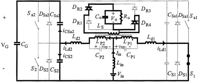
Fig. 13. Second operation stage ( $t_1, t_2$ ).
