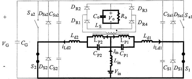
Fig. 12. First operation stage ( $t_0, t_1$ ).
