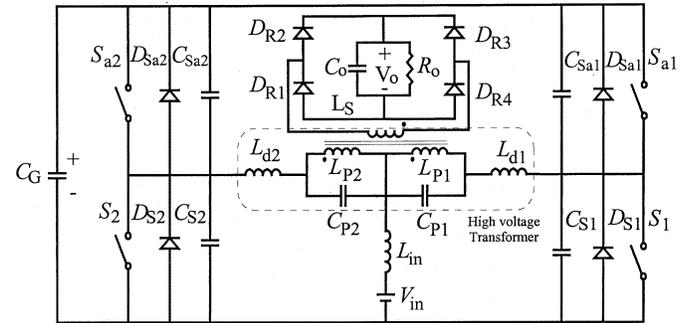
Fig. 11. Proposed power circuit of the single-stage topology.
