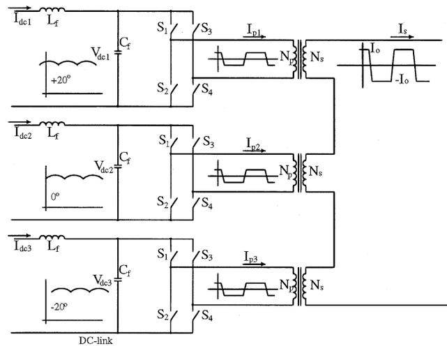
Fig. 8. Circuit to achieve balanced dc-link currents.
