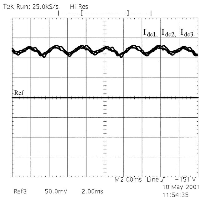
Fig. 11. Balanced dc-link currents. Scales: 2 ms/div, 5 A/div.
