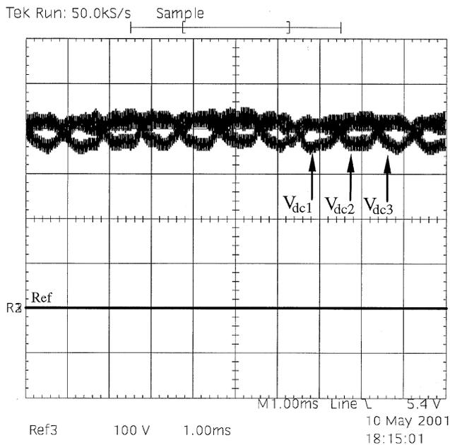
Fig. 13. Rectified voltages through dc-links. Scales: 1 ms/div, 100 V/div.
