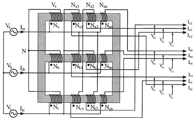
Fig. 2. Scheme of the autotransformer windings.
