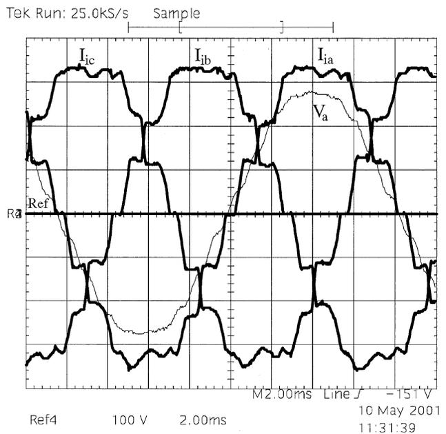
Fig. 15. Line currents. Scales: 2 ms/div, 10 A/div, 100 V/div.
