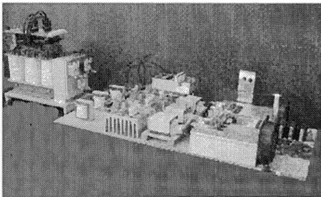
Fig. 9. Prototype of the proposed 12 kW ac-dc converter.
