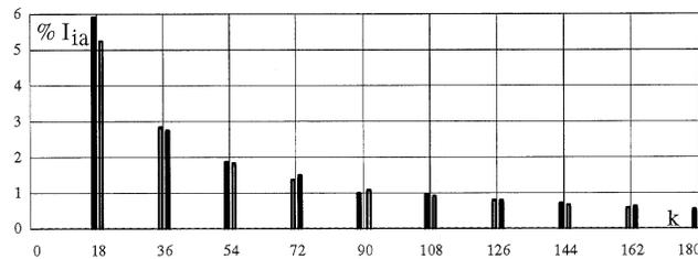
Fig. 7. Harmonics of line current  $I_{ia}$ .
