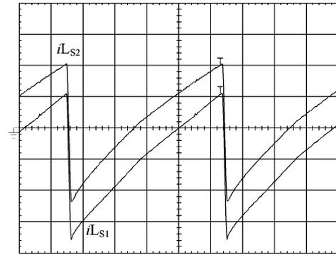
Fig. 10. Current through  $L_{S1}$  and  $L_{S2}$ . (5 A/div, 10  $\mu$ s/div).
