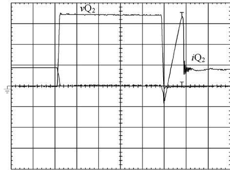
Fig. 8. Voltage and current in  $Q_2, D_2, C_2$ . (100 V/div, 5 A/div, 1  $\mu$ s/div).
