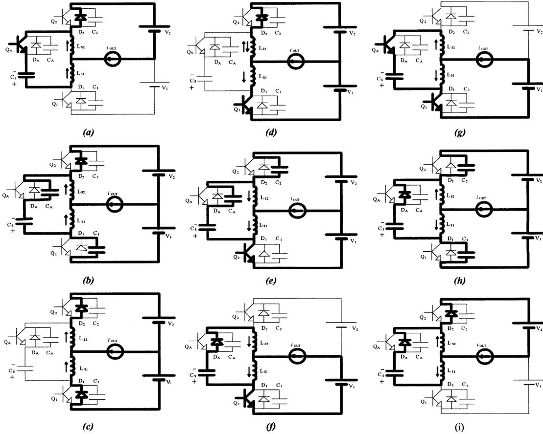
Fig. 2. Operation stages. (a) First state ( $t_0$ - $t_1$ ). (b) Second stage ( $t_1$ - $t_2$ ). (c) Third stage ( $t_2$ - $t_3$ ). (d) Fourth stage ( $t_3$ - $t_4$ ). (e) Fifth stage ( $t_4$ - $t_5$ ). (f) Sixth stage ( $t_5$ - $t_6$ ). (g) Seventh stage ( $t_6$ - $t_7$ ). (h) Eighth stage ( $t_7$ - $t_8$ ). (i) Ninth stage ( $t_8$ - $t_9$ ).
