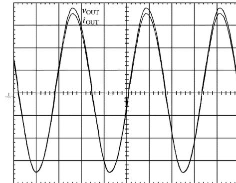
Fig. 12. Output voltage and current. (50 V/div, 5 A/div, 5 ms/div).
