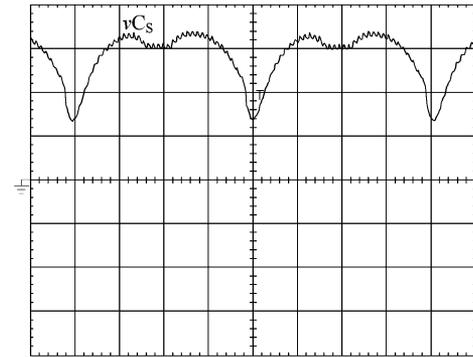
Fig. 11. Voltage in  $C_S$ . (2 V/div, 2 ms/div).
