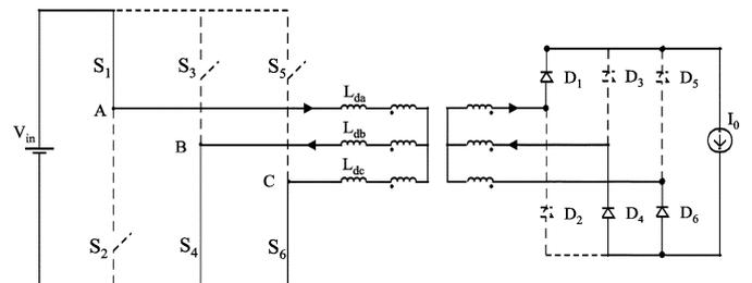
Fig. 9. Third stage for switch  $S_5$   $[t_2, t_3]$ .
