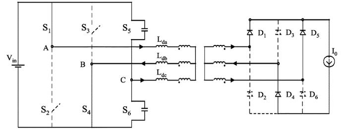
Fig. 7. First stage for switch  $S_5$  [ $t_0, t_1$ ].
