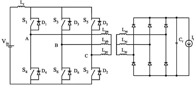
Fig. 4. Three-phase resonant dc link dc/dc converter [6].
