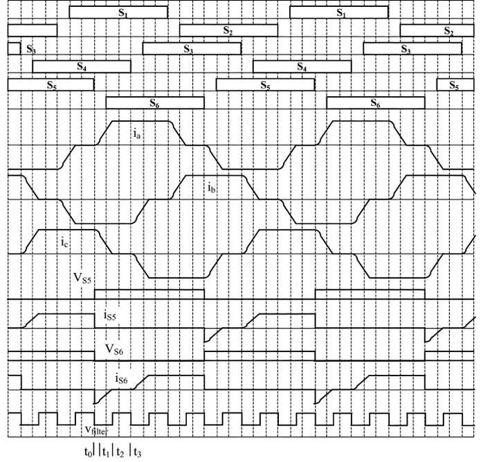
Fig. 6. Main waveforms in the MAXCIM mode.
