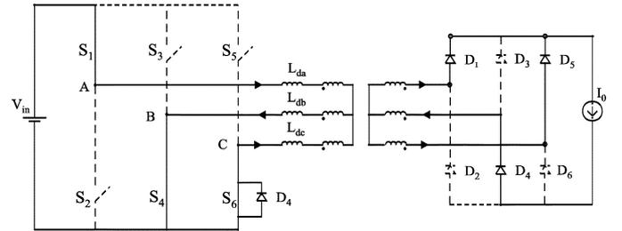
Fig. 8. Second stage for switch  $S_5$  [ $t_1, t_2$ ].
