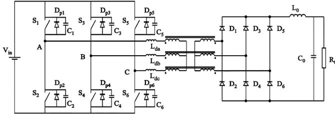
Fig. 5. ZVS dc/dc three-phase converter.
