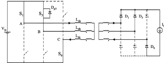
Fig. 19. Fourth stage in VARCIM mode  $[t_3, t_4]$ .
