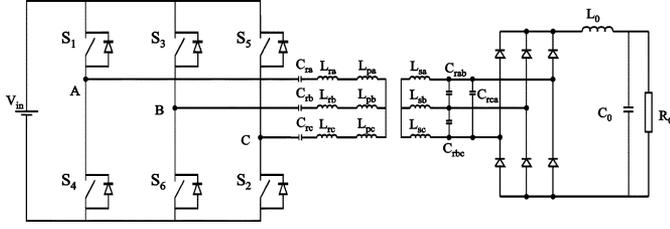
Fig. 3. Three-phase LCC resonant dc/dc converter [5].
