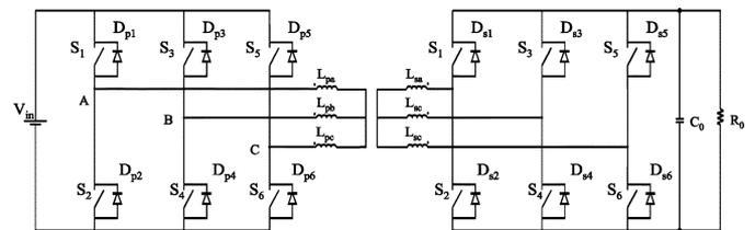
Fig. 2. Three-phase ZVS dc/dc converter [4].
