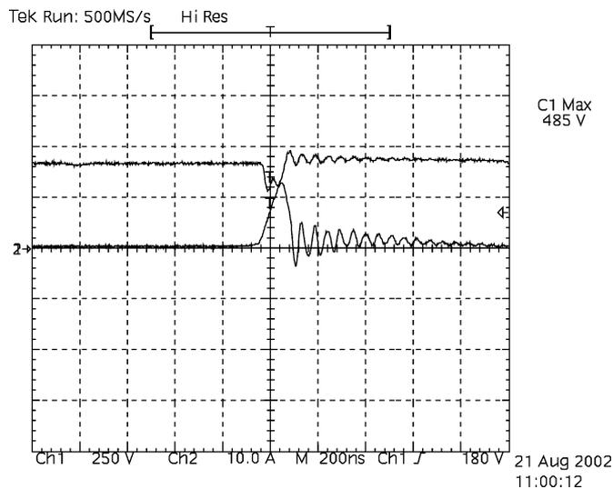
Fig. 22. Detailed view of current and voltage on switch  $S_6$  and capacitor  $C_6$  during turning off ( $C_1 = \dots = C_6 = 1$  nF).
