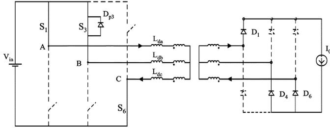
Fig. 18. Third stage in VARCIM mode  $[t_2, t_3]$ .
