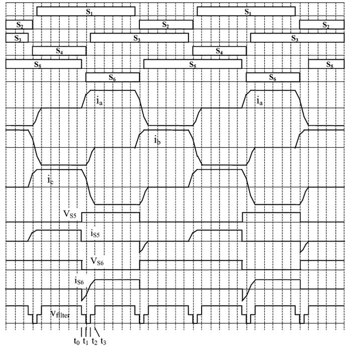
Fig. 15. Main waveforms in the VARCIM mode.
