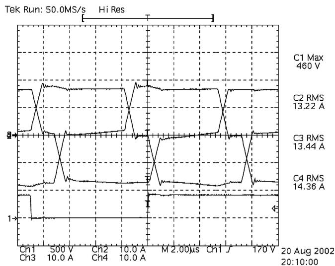
Fig. 23. Currents in the transformer primary side and voltage on switch  $S_6$ .
