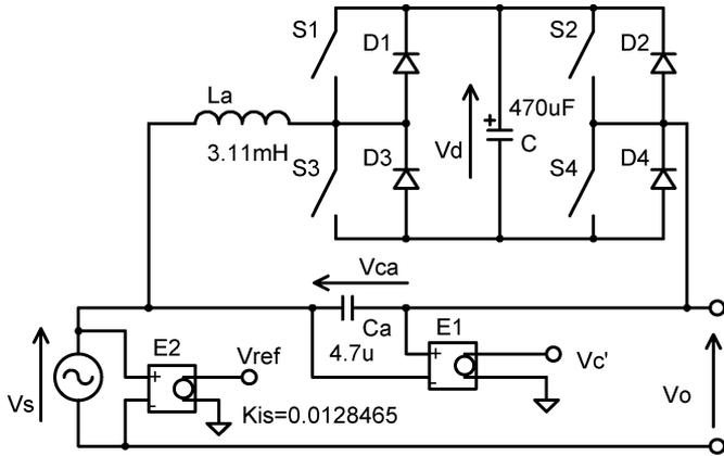
Fig. 7. Simulated power stage circuit.
