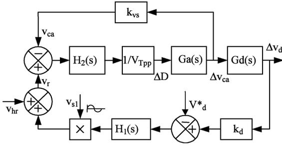
Fig. 6. Control structure of the series active filter.
