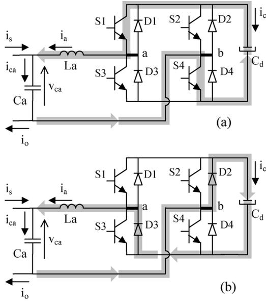
Fig. 5. Active filter operating stages for a switching period.
