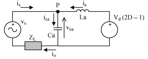
Fig. 4. Equivalent circuit model to the VSI.
