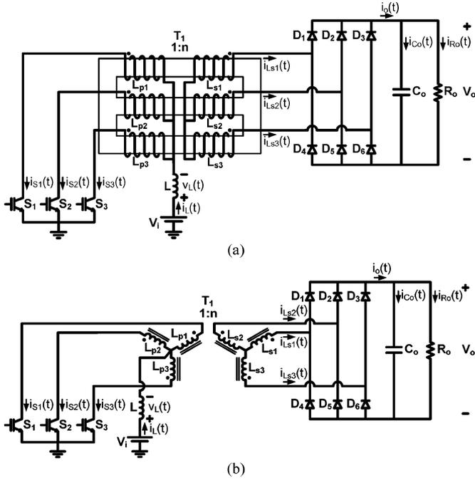
Fig. 1. Circuit of the proposed three-phase current-fed push-pull dc-dc converter. (a) Physical construction of the transformer. (b) Schematic symbol of the transformer.
