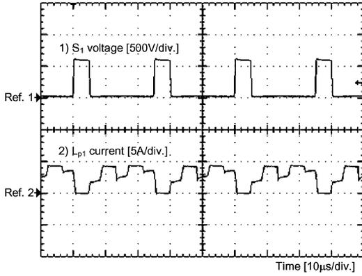
Fig. 13. Voltage across  $S_1$  and current through  $L_{p1}$  for  $D = 0.8$ .
