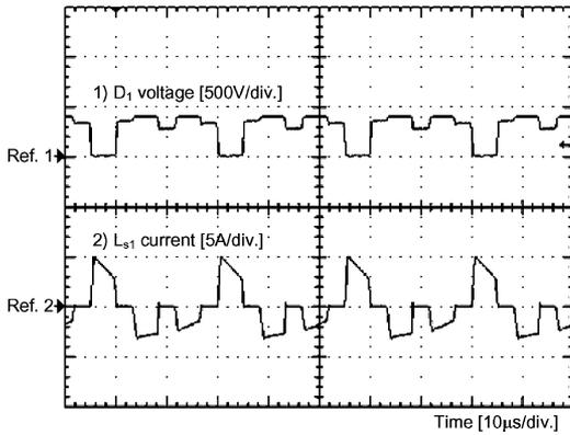
Fig. 14. Voltage across  $D_1$  and current through  $L_{s1}$  for  $D = 0.8$ .
