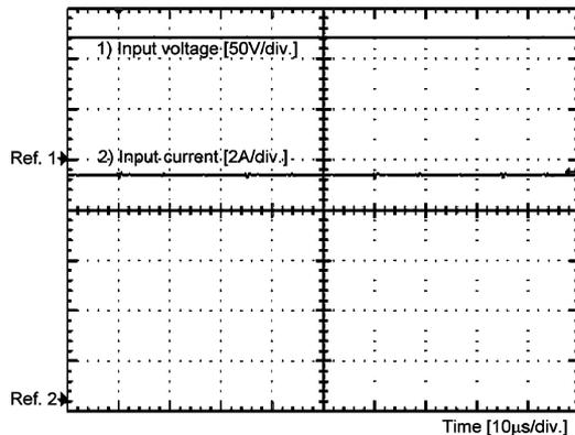
Fig. 21. Input voltage and input current for  $D = 2/3$ .
