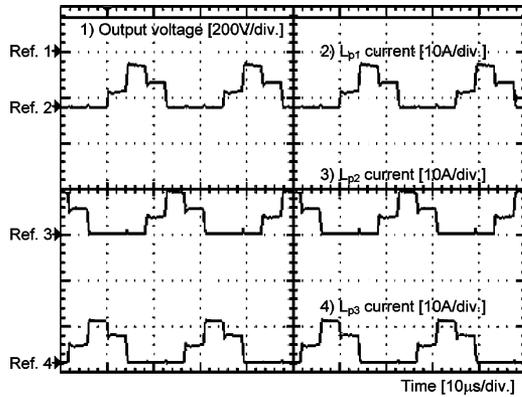
Fig. 19. Output voltage and currents through  $L_{p1}$ ,  $L_{p2}$ , and  $L_{p3}$  for  $D = 0.5$ .
