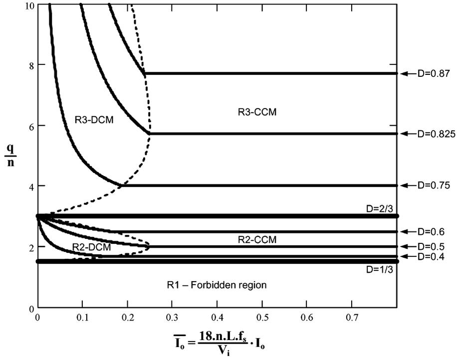
Fig. 10. Output characteristic of the proposed converter.
