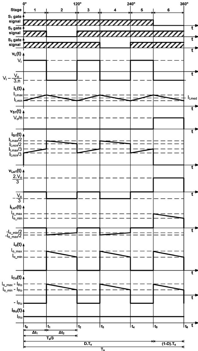
Fig. 7. Main theoretical waveforms for CCM operation in region R3.
