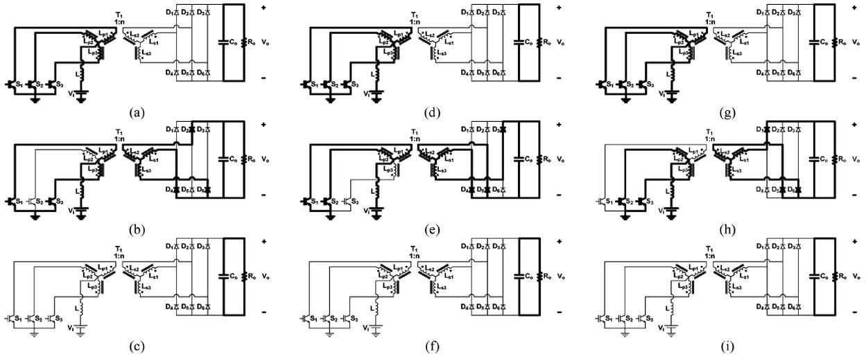
Fig. 8. Topological stages for DCM operation in region R3. (a) First stage ( $t_0, t_1$ ). (b) Second stage ( $t_1, t_2$ ). (c) Third stage ( $t_2, t_3$ ). (d) Fourth stage ( $t_3, t_4$ ). (e) Fifth stage ( $t_4, t_5$ ). (f) Sixth stage ( $t_5, t_6$ ). (g) Seventh stage ( $t_6, t_7$ ). (h) Eighth stage ( $t_7, t_8$ ). (i) Ninth stage ( $t_8, t_9$ ).
