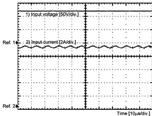
Fig. 20. Input voltage and input current for  $D = 0.5$ .
