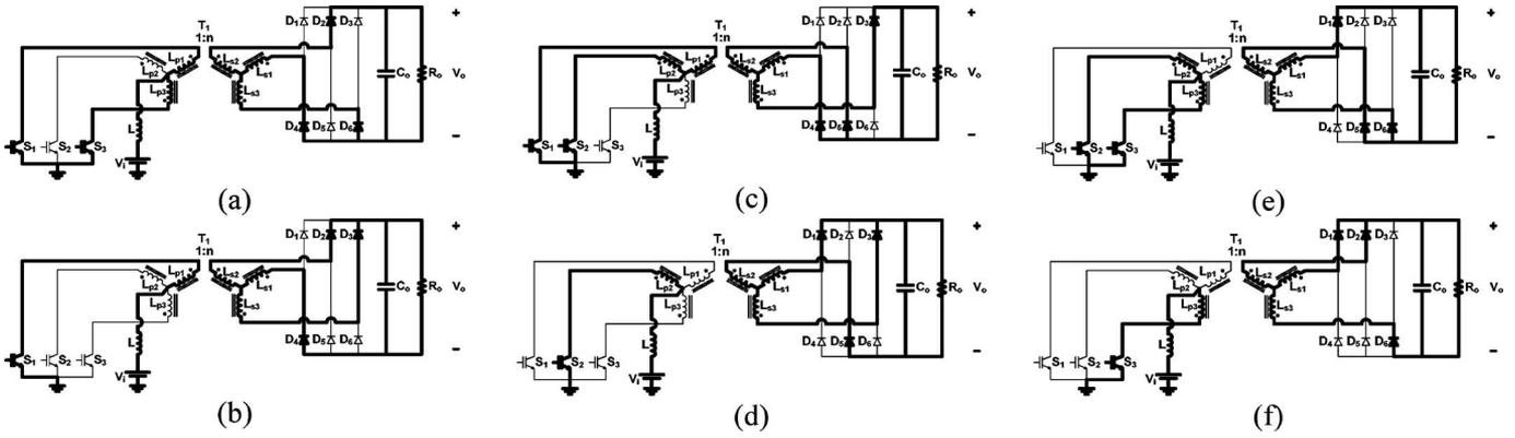
Fig. 2. Topological stages for CCM operation in region R2. (a) First stage ( $t_0, t_1$ ). (b) Second stage ( $t_1, t_2$ ). (c) Third stage ( $t_2, t_3$ ). (d) Fourth stage ( $t_3, t_4$ ). (e) Fifth stage ( $t_4, t_5$ ). (f) Sixth stage ( $t_5, t_6$ ).
