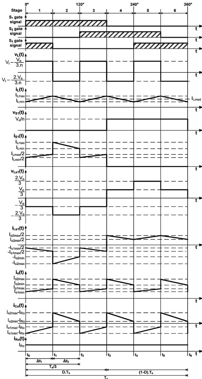
Fig. 3. Main theoretical waveforms for CCM operation in region R2.
