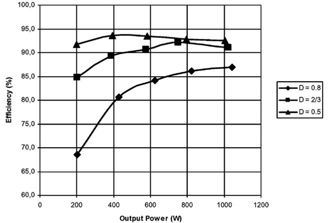
Fig. 22. Converter efficiency as a function of the output power for  $D = 0.5$ ,  $D = 2/3$ , and  $D = 0.8$ .
