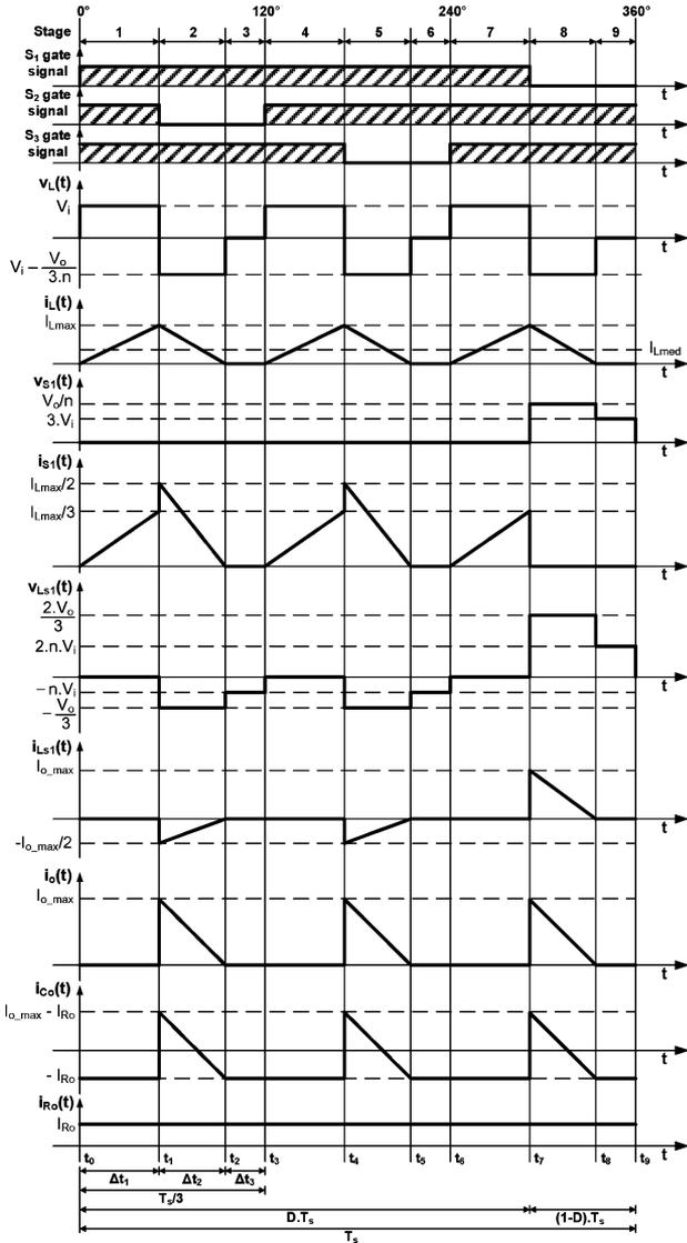
Fig. 9. Main theoretical waveforms for DCM operation in region R3.
