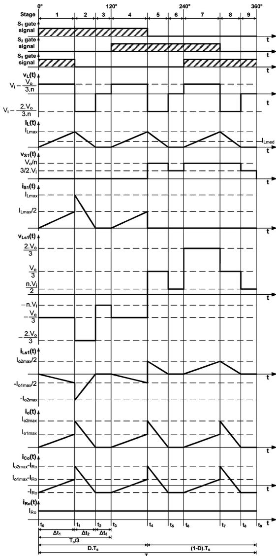
Fig. 5. Main theoretical waveforms for DCM operation in region R2.
