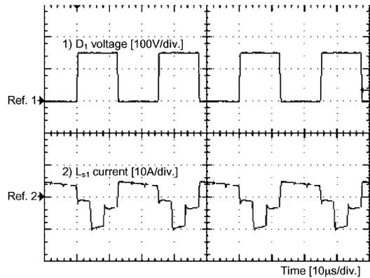
Fig. 18. Voltage across  $D_1$  and current through  $L_{s1}$  for  $D = 0.5$ .
