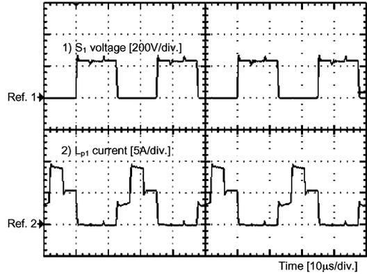
Fig. 17. Voltage across  $S_1$  and current through  $L_{p1}$  for  $D = 0.5$ .
