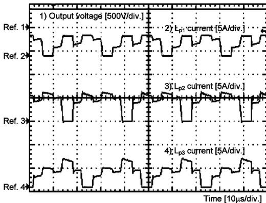
Fig. 15. Output voltage and currents through  $L_{p1}$ ,  $L_{p2}$ , and  $L_{p3}$  for  $D = 0.8$ .
