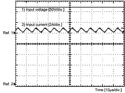
Fig. 16. Input voltage and input current for  $D = 0.8$ .
