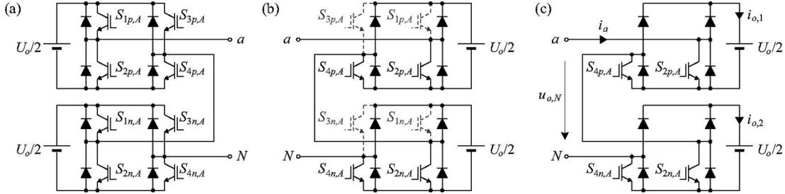
Fig. 2. Derivation of a unidirectional rectifier based on the (a) five-level cascaded H-bridge inverter [23], [24]. (b) Switches  $S_{1p,A}$ ,  $S_{3p,A}$ ,  $S_{1n,A}$ , and  $S_{3n,A}$  are not required for rectifier only operation. (c) Leg of the cascaded H-bridge-based PWM rectifier topology.
