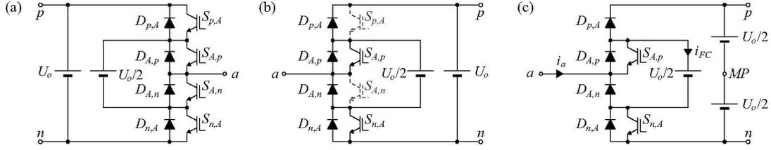
Fig. 1. Derivation of a unidirectional rectifier based on the (a) three-level flying capacitor inverter [21], [22]. (b) Switches  $S_{p,A}$  and  $S_{A,n}$  are not required for rectifier only operation. (c) Leg of the FC-based PWM rectifier topology.
