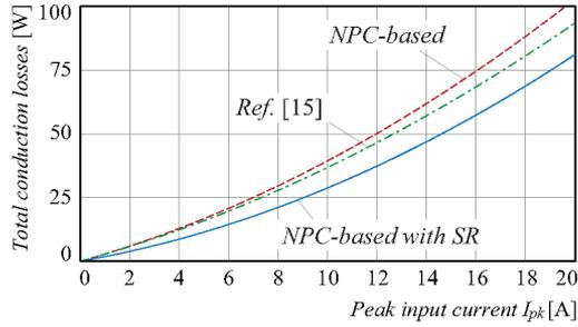
Fig. 7. Total conduction losses for the three-phase/three-level rectifier proposed in [15] and for the NPC-based [cf., Fig. 3(c)] with and without synchronous rectification for  $M = 0.78$ .
