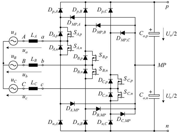
Fig. 5. The three-phase/level NPC-based PWM rectifier.
