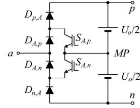
Fig. 6. Three-phase/three-level rectifier proposed in [15].
