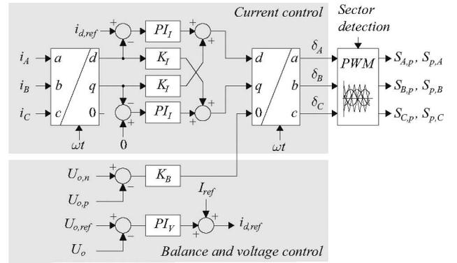
Fig. 8. Control simulation model for verifying PFC operation.
