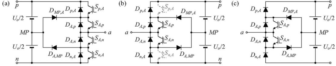
Fig. 3. Derivation of an unidirectional rectifier based on the (a) three-level NPC inverter [25]. (b) Switches  $S_{p,A}$  and  $S_{n,A}$  are not required for rectifier only operation. (c) Leg of the NPC-based PWM rectifier topology.
