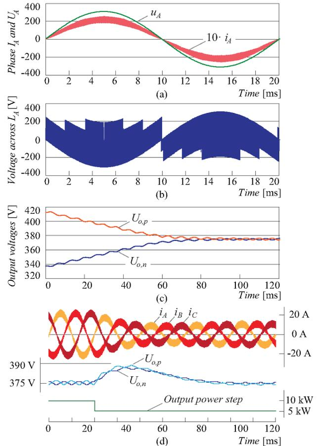
Fig. 9. Simulation results for verifying PFC operation. (a) Phase A input current  $i_A$  and voltage  $u_A$ . (b) Voltage across the input inductor  $L_A$ . (c) Output voltages  $U_{o,p}$  and  $U_{o,n}$  development after a 20% unbalance. (d) Input currents, output voltages and power for a load step from 10 to 5 kW.
