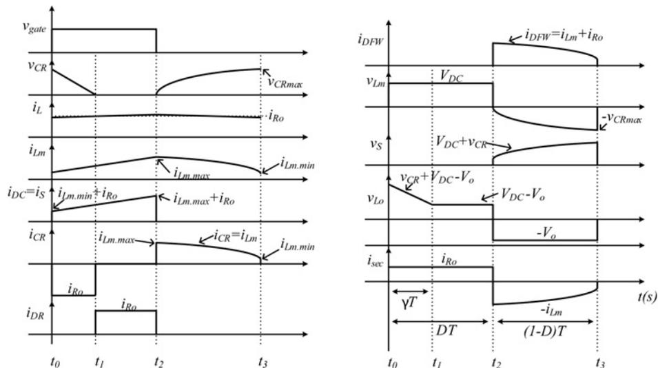
Fig. 3 Resonant reset forward converter waveforms
