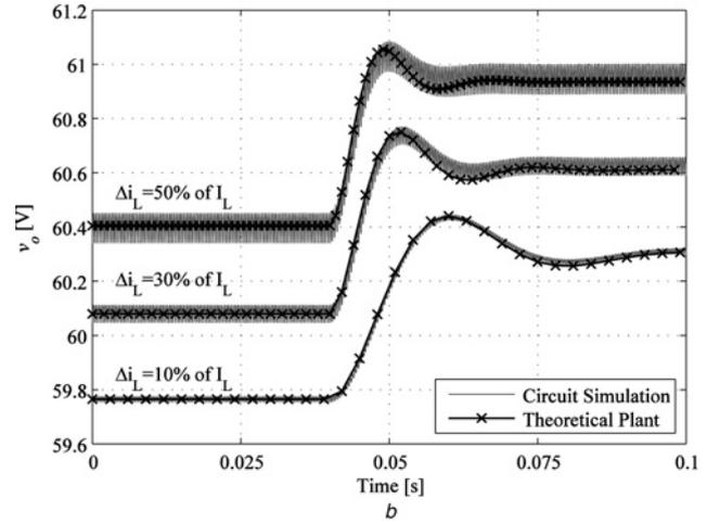
**Fig. 5** Simulation with three different current ripples
