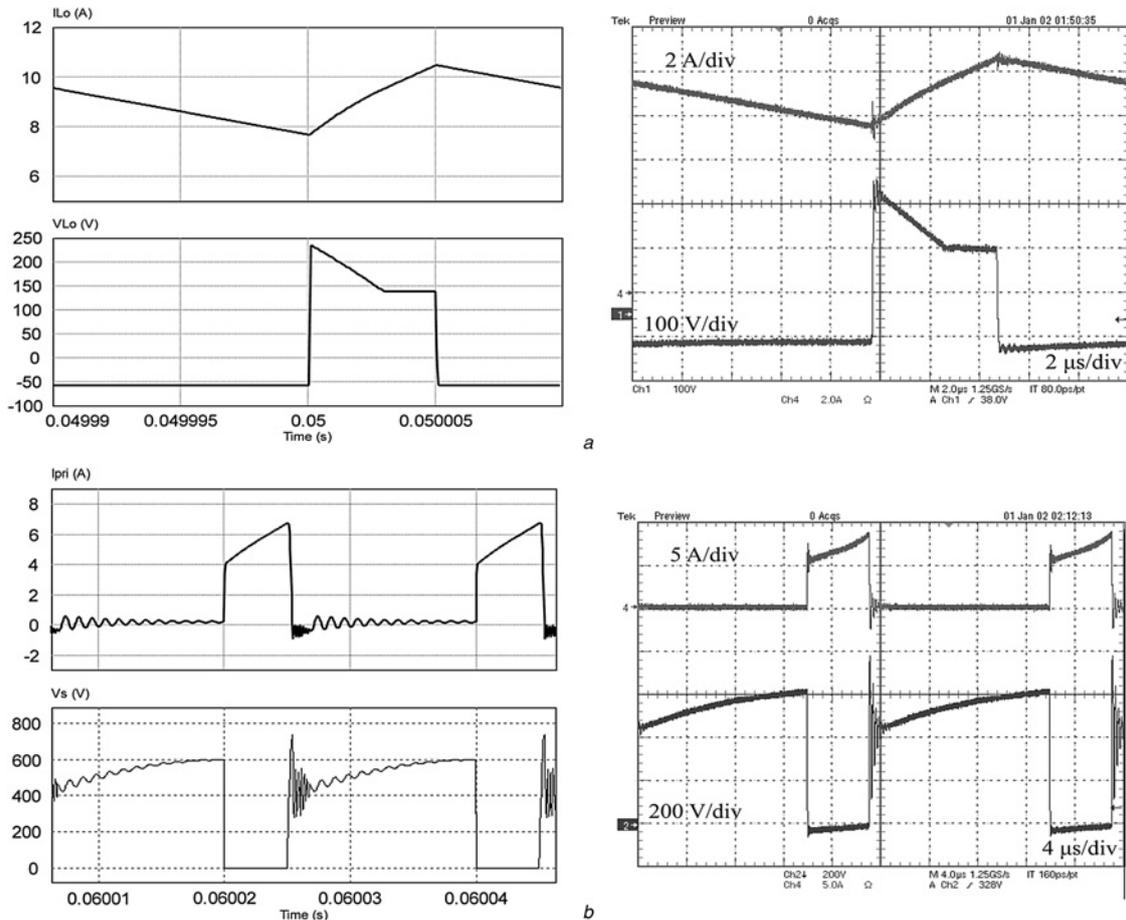
**Fig. 7** Simulation and experimental results for the resonant reset forward converter
