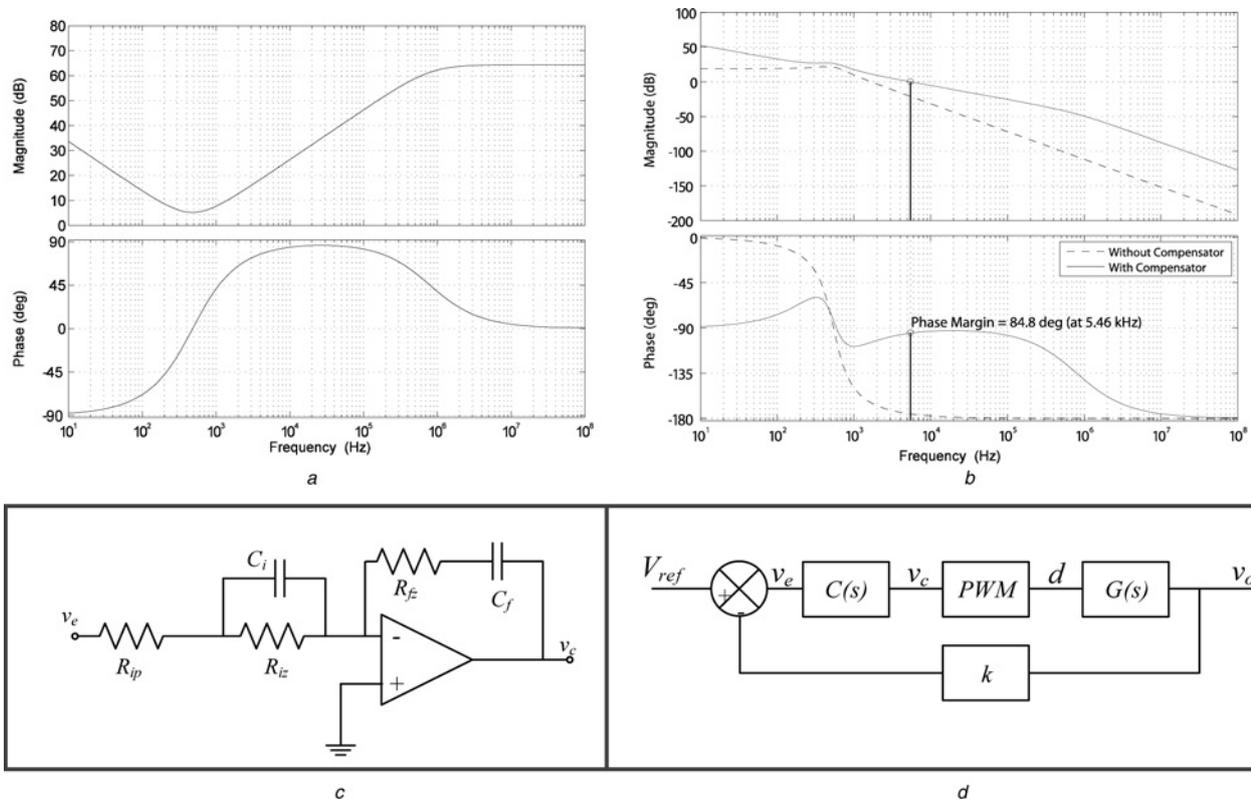
**Fig. 6** Theoretical frequency responses (amplitude and phase) of the converter plant
