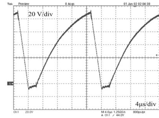
Fig. 8 Simulation and experimental results for the resonant reset forward converter
