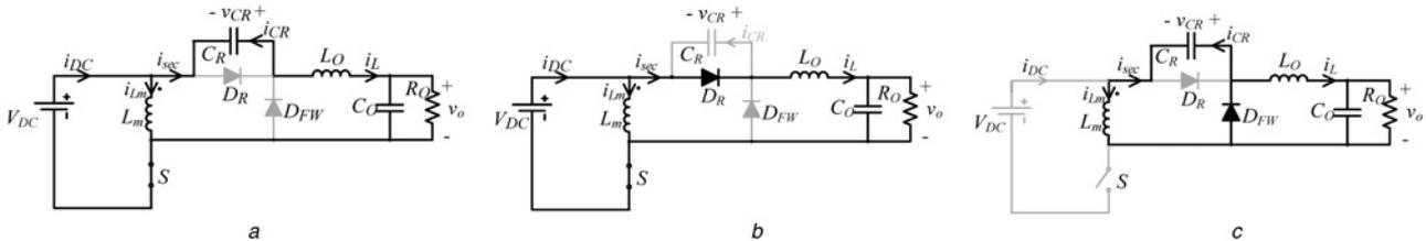
Fig. 2 Topological stages of the resonant reset forward converter
