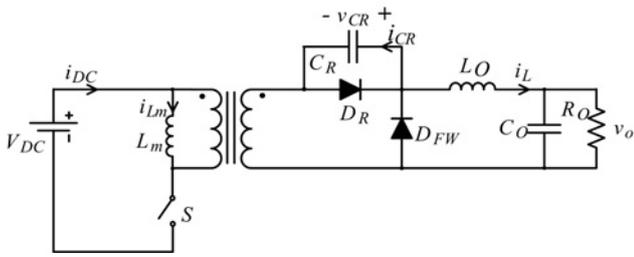
Fig. 1 Forward converter with resonant reset at the secondary side
