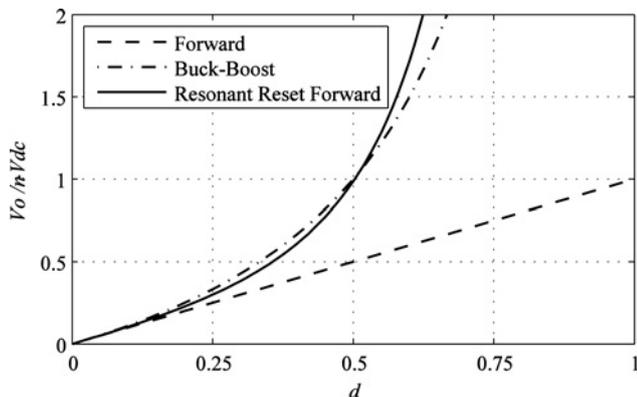
Fig. 4 Converter output characteristics
