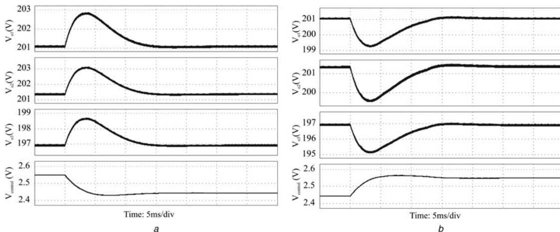
**Fig. 10** Load transient response
