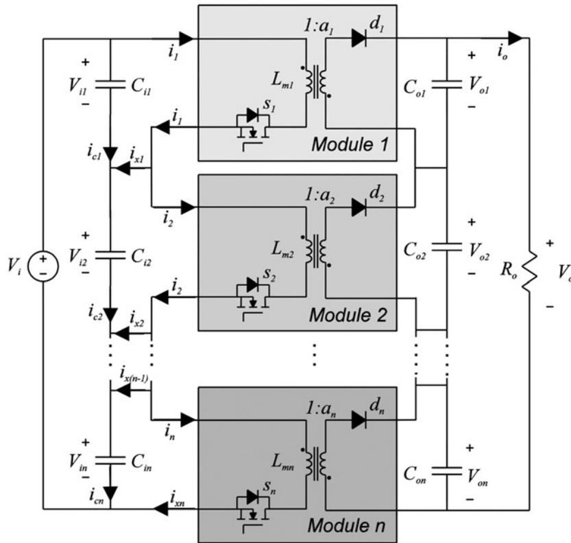
Fig. 1 Flyback converters in ISOS connection
