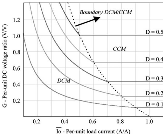
**Fig. 3** Static output characteristics of the flyback converter
