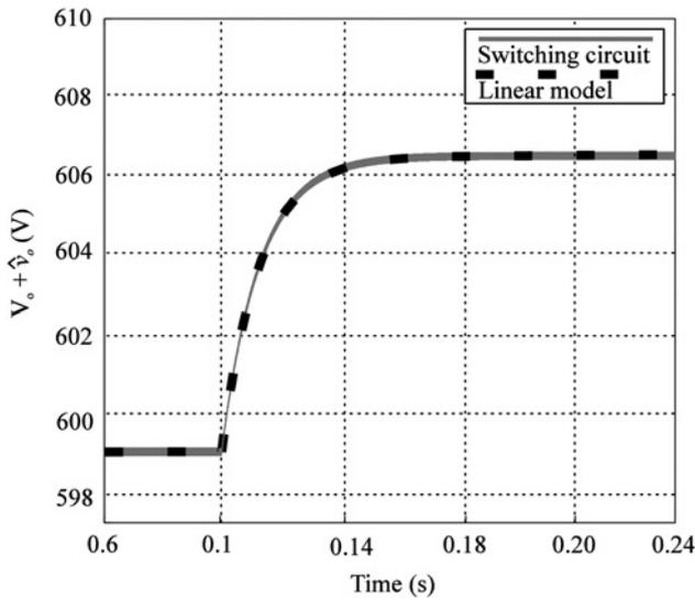
Fig. 7 Open-loop response of output voltage to step change in duty cycle
