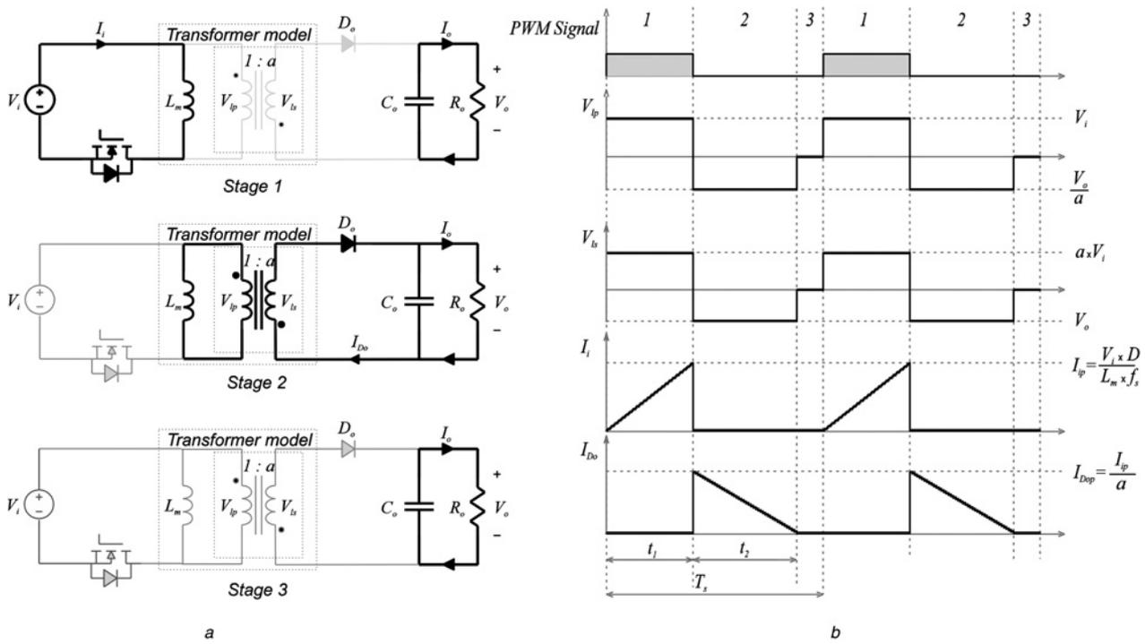
**Fig. 2** Flyback converter in DCM operation
