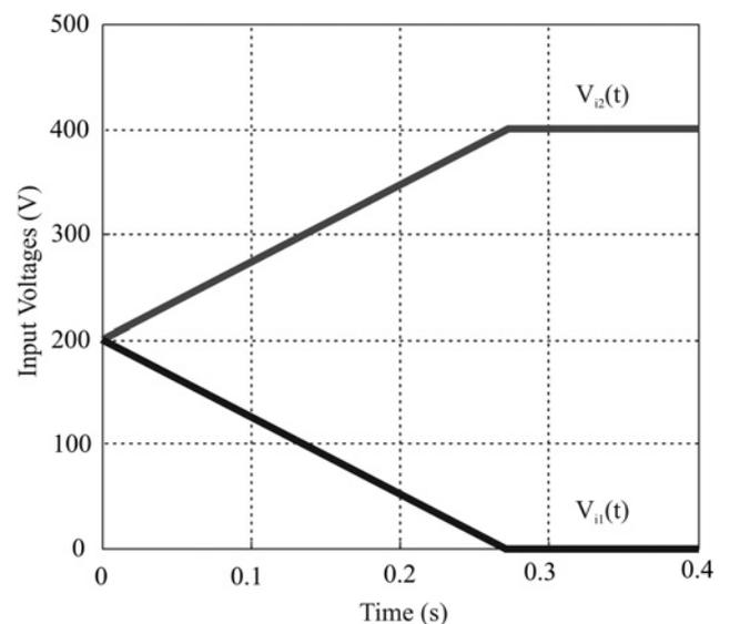
**Fig. 6** Input-voltage behaviour from simulation results
