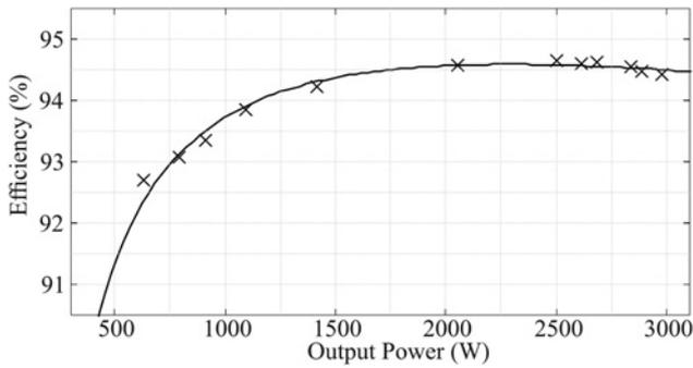
**Fig. 11** Measured efficiency of DCM flyback converter in ISOS connection with three modules
