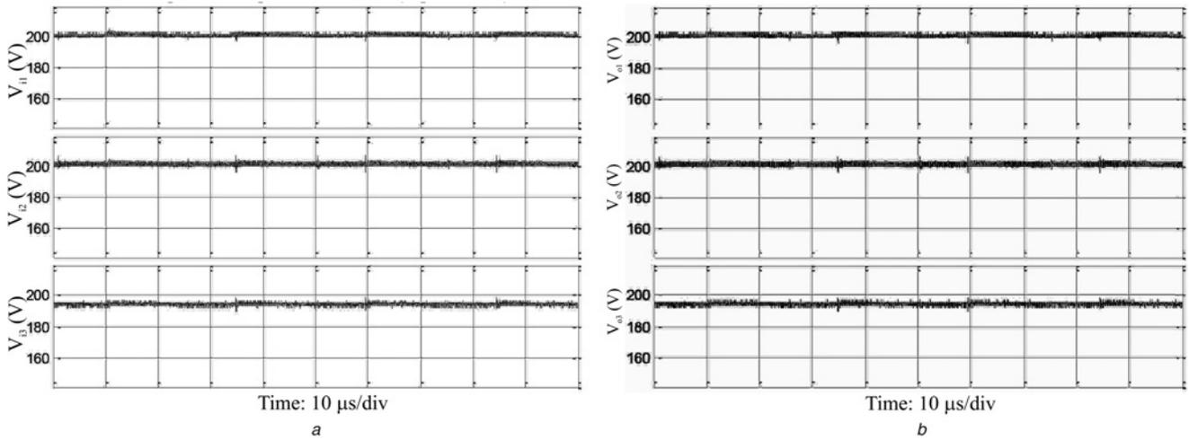
**Fig. 9** Voltage-sharing between the modules in steady-state operation
