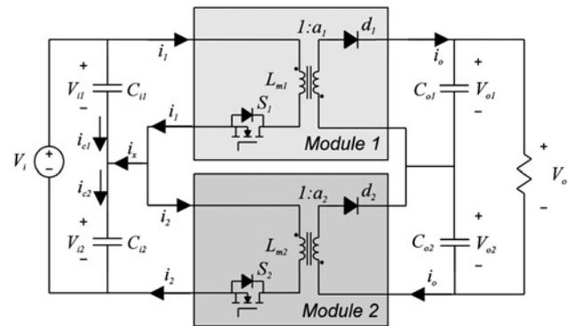
**Fig. 5** Two flyback converters in ISOS connection
